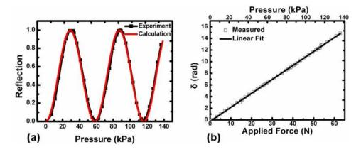
Assuming the fiber is fully elastic and mechanically homogeneous, the photoelastic phase retardation induced by the applied force is given by [19]:
