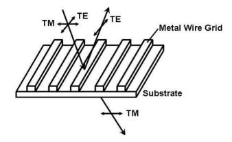
Figure 1. The working principle of a wire grid polarizer.
