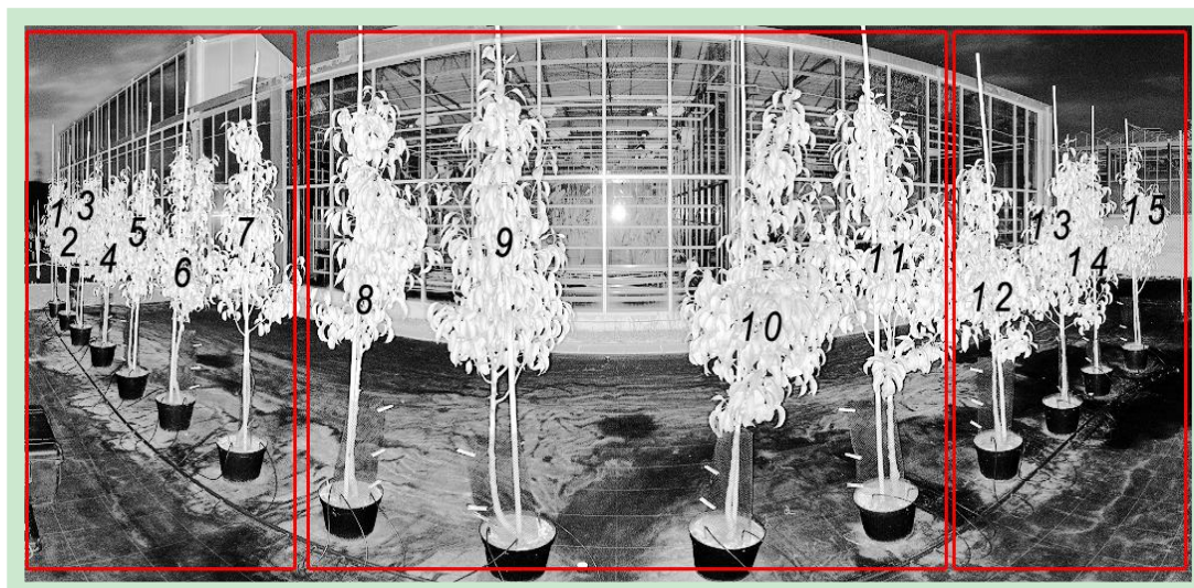
Figure 2. Part of a hemispherical projection of a TLS scan of 15 two years old pear trees (first row). The corrected intensity and angle of incidence relationship is tested on leaves of those trees. Trees are grouped by their distance to the beam aperture (red frames).
