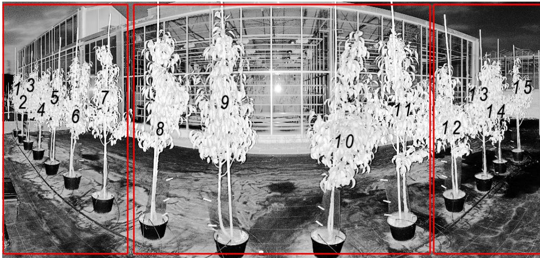
Figure 2. Part of a hemispherical projection of a TLS scan of 15 two years old pear trees (first row). The corrected intensity and angle of incidence relationship is tested on leaves of those trees. Trees are grouped by their distance to the beam aperture (red frames).
