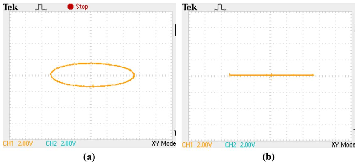
This in phase term which is due to frequency split will be difficult to eliminate from the useful Coriolis force without considering other factors. However, since a frequency split will result in a quadrature error which could be separately observed, its feedback to eliminate the frequency split can finally eliminate the in phase error term brought about by the frequency split.
