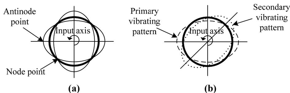
The math model proposed by Lynch is used in this paper with the resonator operating in the  $n = 2$  mode [17,18]. In the math model, mass and stiffness imperfections causing frequency split between the two modes and inhomogeneous damping dependent on the circumference angle are considered. The equations are presented as follows:
