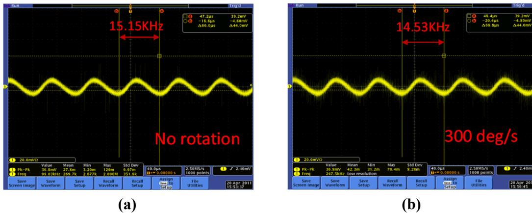
**Figure 8.** Sensitivity evaluation of the fabricated SAW gyroscope.
