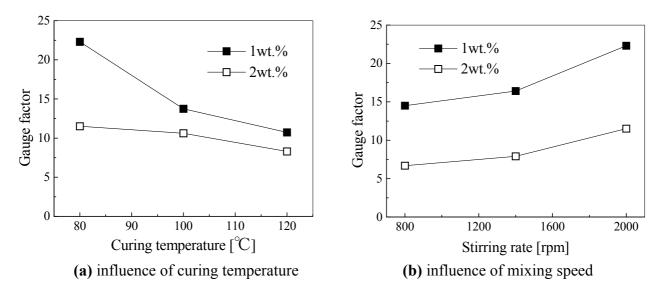
Figure 12. Influences of mixing speed and curing temperature on sensor sensitivity.
