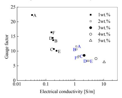
Figure 13. Relationship between electrical conductivity and sensor sensitivity.
