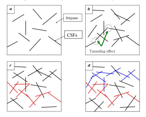
Figure 1. Percolation process in conductive composites.
