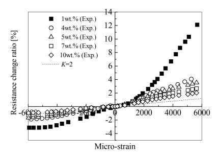
Figure 15. Piezoresistivity of sensor using MWNT-7.
