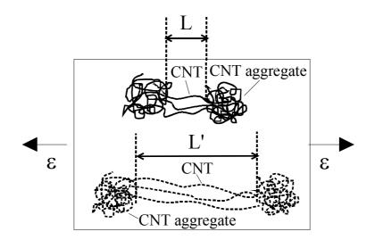
When subjected to applied strains, these bridging CNTs will elongate (e.g., from L to L' in Figure 19 after elongation) or contract depending on the tensile or compressive strains. Therefore, as reported in many studies [25,81,82], the resistance of CNTs themselves will linearly change, which leads to the
