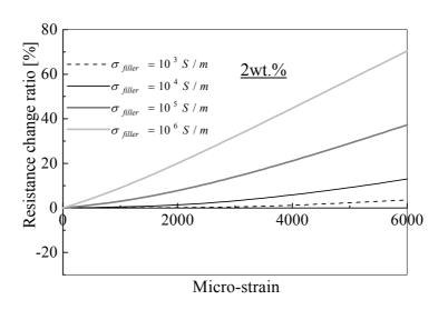
Figure 24. Influence of electrical conductivity of filler on sensor sensitivity.
