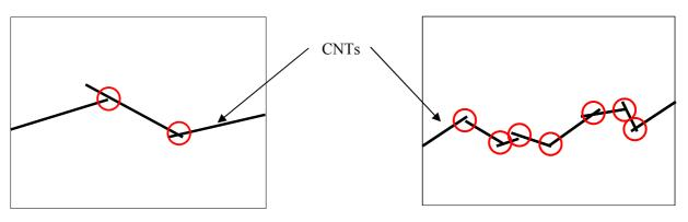
Figure 20. Influence of aspect ratio of fillers on conductive network.
