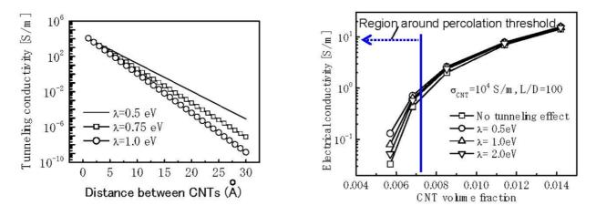
(a) Tunneling conductivity for various distances (b) Effect of tunneling effect on conductivity
