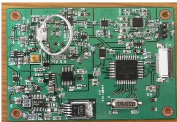
The data processing block is operated by a microcontroller PIC18F452 with a built-in 10-bit A/D converter. Figure 3 shows the prototype of the UHF RFID reader, and Table 1 presents the design details.
