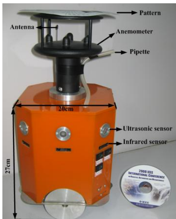
Figure 8. The small mobile MrCollie robot and onboard sensors.
