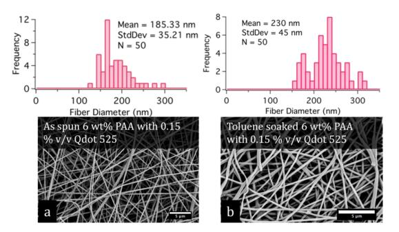
Figure 9. SEM micrographs of composite mats (a) as spun and (b) after soaking in toluene.
