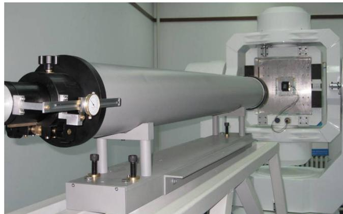
The sun simulator can send a parallel light beam and the rotating platform can provide different incident sunray angles with a position accuracy of  $0.001^\circ$ . The performance test indicates that the FOV of the sun sensor is larger than  $\pm 60^\circ \times \pm 60^\circ$ , and the maximum error between the measured sun position in the form of incident angle and the setting position through the rotary table is less than 0.08 degrees of arc (see Figure 13 for the half FOV statistics).
