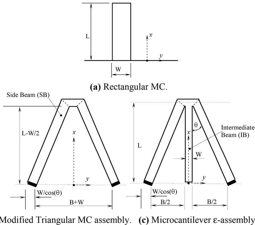
For a concentrated force exerted on the rectangular microcantilever tip ( $x = L$ ), the solution of Equation (1), denoted by  $z_{aF}(x)$ , subject to boundary conditions given by Equation 3(a,b) can be expressed as:
