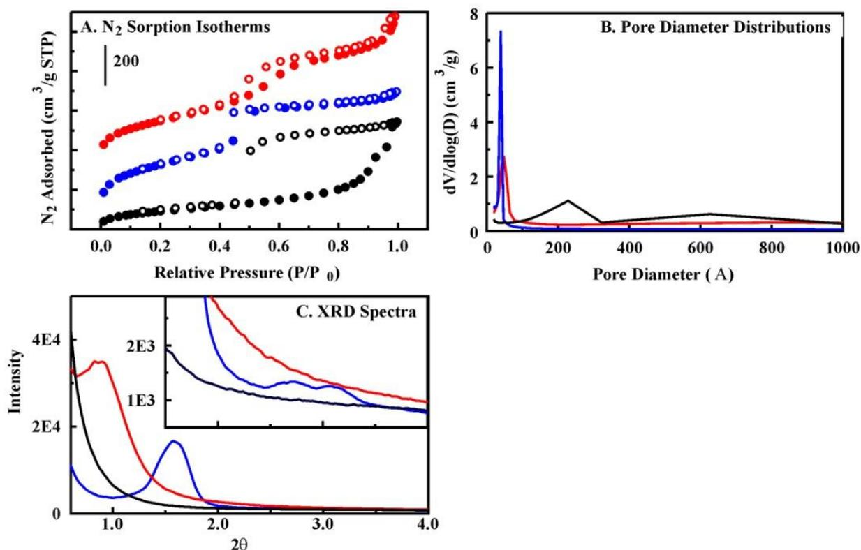
A similar balance in characteristics can be noted for the other materials considered. The large hysteresis in the nitrogen sorption isotherm for OTS and its broad pore size distribution indicate complexity in the pore structure of that material related to pore shape and/or interconnectivity [22]. Lack of mesoscale order in OTS was also confirmed by the absence of reflections in its powder XRD
