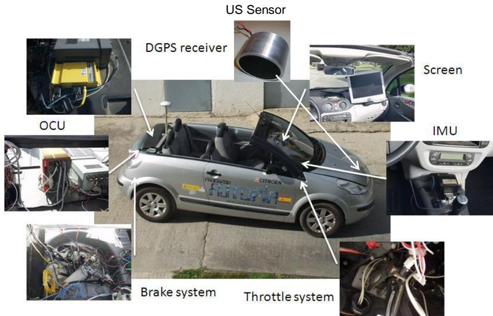
Regarding the throttle pedal, a potentiometer converts the pressure applied on the pedal by the driver into an analog signal that can be read by the vehicle's control unit. For its automation, the signal coming from the potentiometer was cut and a switch was installed in order to choose between the analog signal coming from the potentiometer (via the throttle pedal) or the signal coming from an analog output card connected to the On-board Control Unit (OCU) which is controlled via software.
