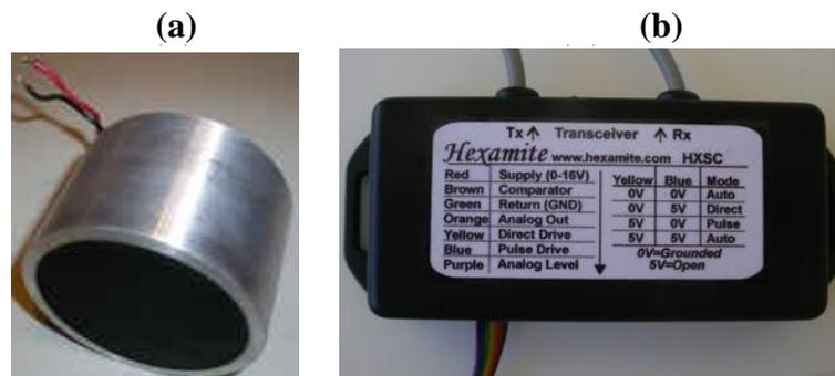
To trigger the ultrasonic sensor and to capture and process the signal received, a laptop equipped with a data acquisition card has been used. Signal processing is performed ten times per second, according to the model described in the previous section. This processing involves several stages:
