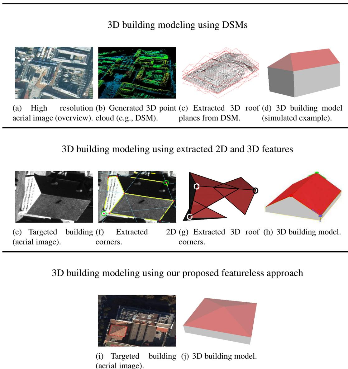
Figure 2 (Top) illustrates the building modeling using Digital Surface Models. Figure 2 (Middle) illustrates the building modeling using reconstructed geometrical features (e.g., 2D vertices and lines). Figure 2 (Bottom) illustrates our proposed featureless approach.
