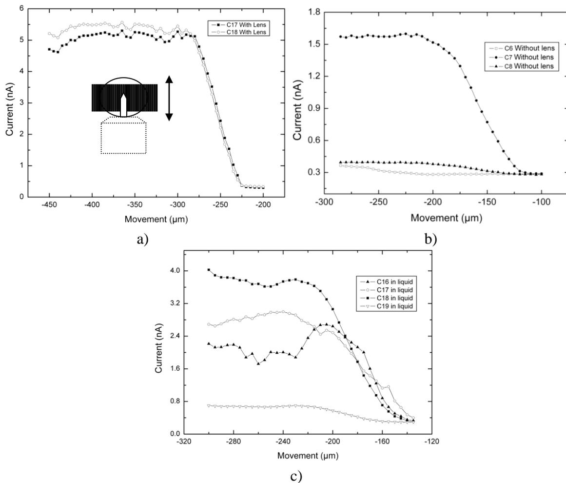
Liquid made it difficult to maintain the focus. In Figure 3(c), the relevant three line sensors or channels (C17, C18, C19), obtain a signal response more than double that given by the noise level. The reason why there is instability coming from the response of at least one detector is because the slightest movement of the liquid was causing at some instances the loss of image focus on the sensor.
