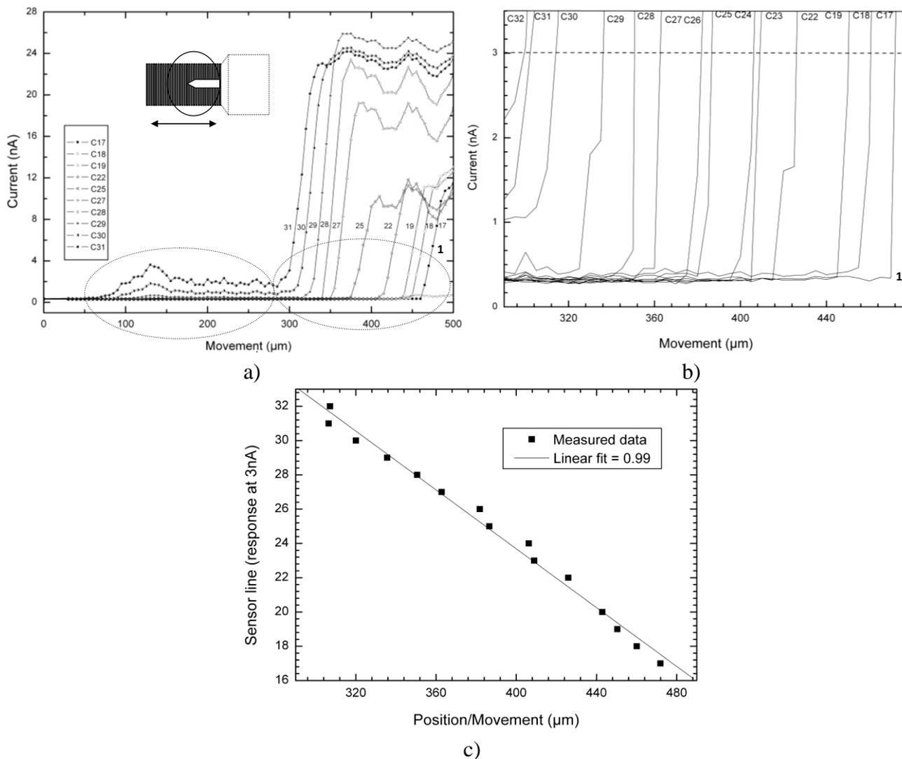
Figure 5(b) shows the response (as a function of position/movement) obtained by all line sensors just for the signal related to the holding structure (not the signal related to the micro cantilever) at the 3 nA line, which cuts across in order to help determining linearity of the sensor in this particular situation, which is next sketched in Figure 5(c).
