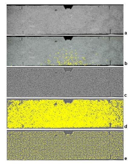
Figure 7 shows the original image of a small beam (a) and the detected corners with the FAST operator (b). As can be seen, few points can be measured. The filtered image (c) provides more corners (d) with a better distribution. At the end of the process points can be mapped (d) onto a "quasi" regular grid (in this case each cell is  $50 \times 50$  pixels roughly).
