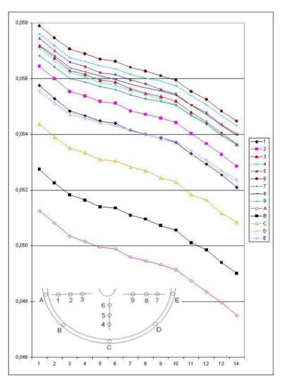
Figure 11. Vertical displacements (at different epochs) measured with the image-based method.
