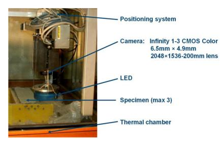
Figure 1. The developed system for crack aperture estimation.
