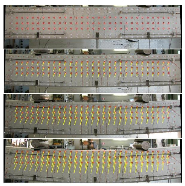
Figure 5. Some rectified images of the sequence and the magnitude of the displacements.
