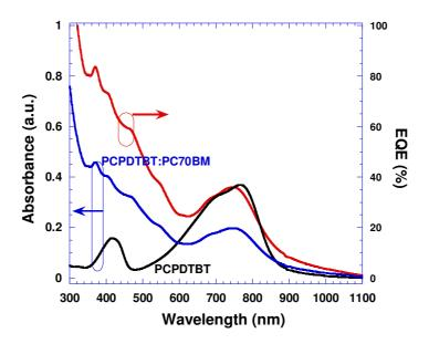
The photo-active layer in our PPDs comprises a phase separated blend of PCPDTBT and PC<sub>70</sub>BM. The two components form interpenetrating donor/acceptor networks in the bulk heretojunction (BHJ) structure. Three different PPD architectures were investigated:
