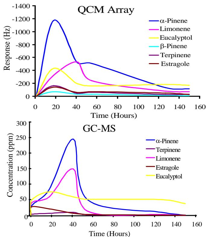
A quite similar emanation behavior was observed from both devices when exposed to fresh and dried herbs. Vapors of terpenes emitted from fresh and dried herbs were transferred through a heated Teflon sample-tube for GC-MS analysis. The data obtained showed that a maximum amount  $\leq 250$
