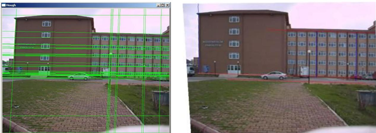
In our acquisition plan, the camera is stable. In this case, when the rectification parameters are found for the first time, they can be used until the camera changes its position. Thus, at the beginning of the speed estimation application, at first the rectification parameters can be found for the first time and these parameters can be used as long as the camera stays stable.
