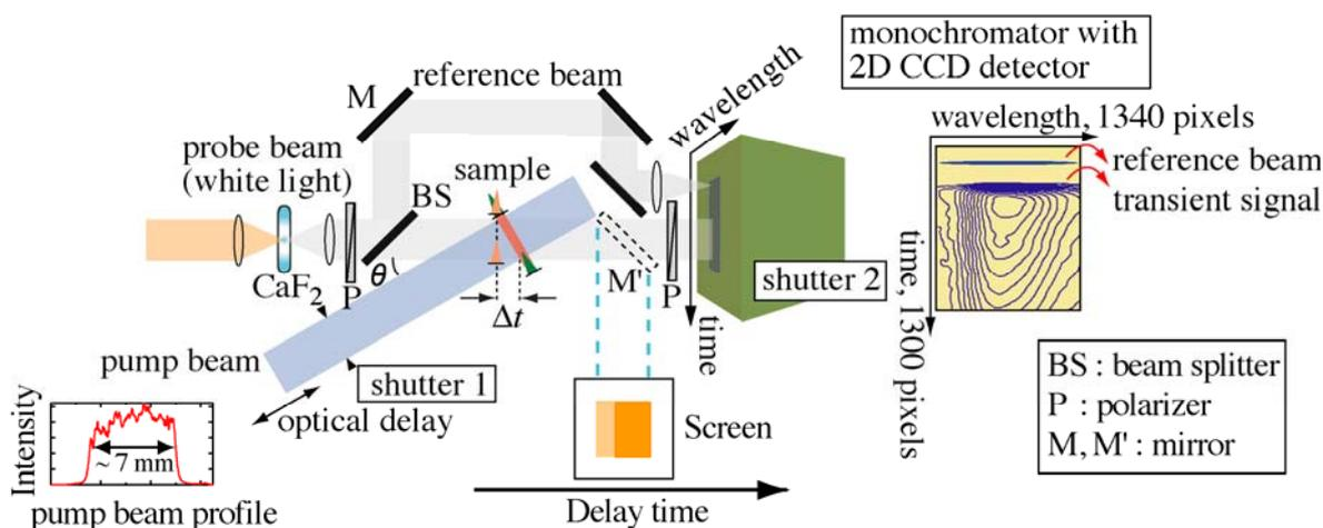
When performing the imaging experiments on film samples, to avoid photodegradation as much as possible without any sample circulating/rotating systems, we insert a solenoid shutter (shutter 1)
