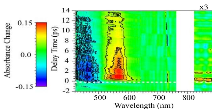
Figure 13 shows the time-resolved absorbance change spectra with different delay times reproduced by slicing off the 2D image shown in Figure 12. As comparison, the experimental data of  $\beta$ -carotene in *n*-hexane solution measured by the conventional pump-probe transient absorption spectroscopy are
