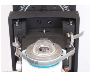
Figure 6. Detail of the system to fasten the radiometer under test on to the automatic arm.
