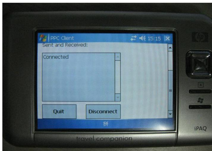
The PDA connects to port 1025 and 1026 of the server, and server receives ECG and temperature data at both of two ports. As the PDA sends 333 ECG sampling data per second, it must send 1,332 bytes per second to server, due to the data being float type.
