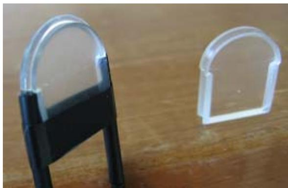
The optimal radius sensor is suitable for sensors which are placed at the top of the battery. For lower positions between the plates, the design of the battery should be adapted properly. When the fiber sensor with the optimal radius is to be introduced inside an operational standard battery, as it was the case in the present project, the process is very difficult or even impossible to implement depending
