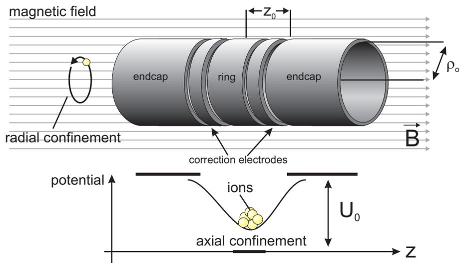
In a so-called “ideal” Penning trap, *i.e.*, in the absence of inhomogeneities and anharmonicities, the axial oscillation frequency of a confined ion is given by
