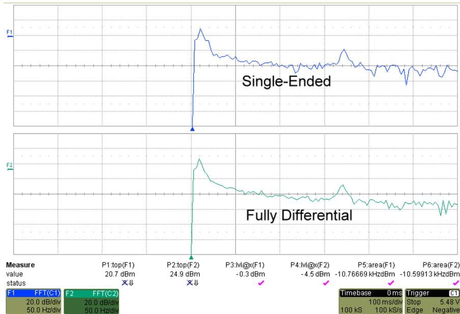
**Figure 16.** Input current *versus* SFDR of SE and FD potentiostat.
