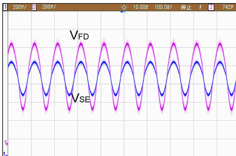
The Fast Fourier transformation is utilized to perform the analysis of the circuit linearity. The sine wave current signal is routed through the input and the corresponding output voltage is recorded and analyzed. By recording the fundamental signal power  $S$  and the strongest harmonic distortion power, which is introduced due to non-linearity in the conversion  $D_2$ , the spurious-free dynamic range SFDR can be calculated as:
