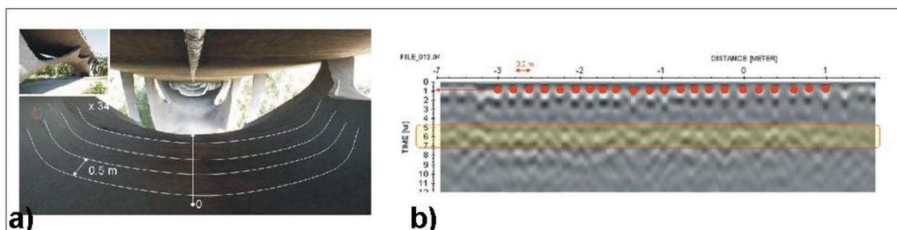
Data processing steps were: trace editing, marker interpolation, time zero correction, header gain removal, ACG gain and fk-filter. Finally, data were migrated with a velocity of 0.06 m/ns estimated by using the hyperbola adaptation method. Although the survey was performed in a dry period, the encountered value of velocity can be indicative of a great moisture content of the concrete. Figure 11 shows an example of raw data obtained on Musmeci bridge, with the time-zero stated at 3.5 ns in order
