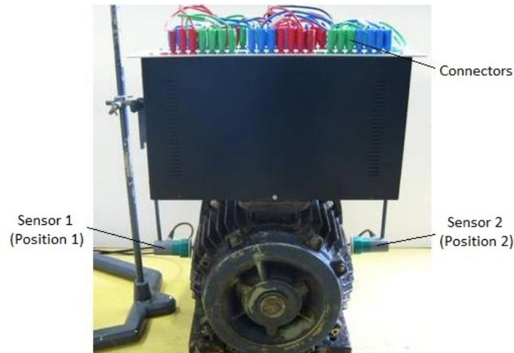
Verification have also be done in order to make sure that the currents in the wires going up from the machine towards the connector block do not disturb the measurements. Positions 1 and 2 correspond respectively to  $\beta_0$  and  $\beta_0 + \pi$  (see paragraph 5.2)  $\beta_0$  are chosen “arbitrarily”.
