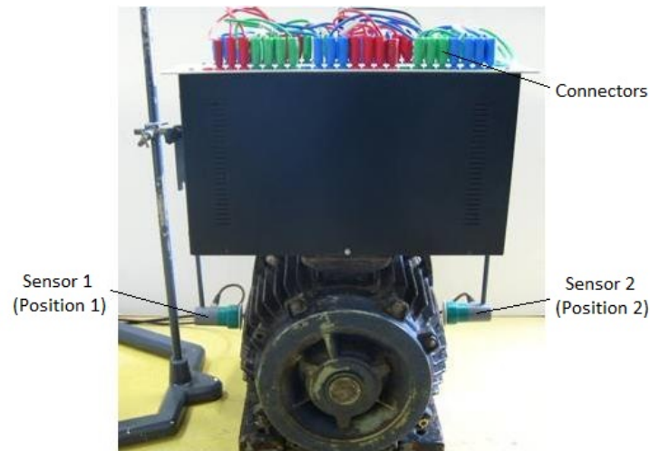
Figure 7. Salient synchronous modified machine and the sensors' positions.
