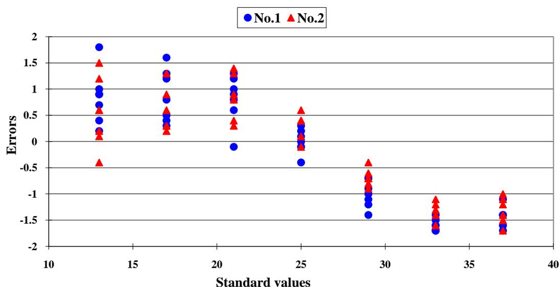
The error distributions of two TROTEC BP-20 infrared thermocouples are presented in Figure 5. When the measurement data of sensor No. 4 was calculated with the calibration equation that was established from sensor No. 3, the predictive errors were higher than 1.2 °C.
