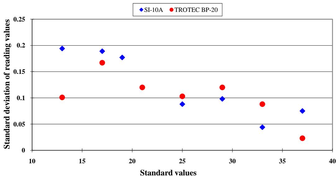
Below the measurement temperature of  $25$  °C, the standard deviations were less than  $0.2$  °C. In the higher temperature range, the standard deviations were less than  $0.1$  °C. From the viewpoint of practical applications, this sensor had good precision performance. The estimated parameters and statistics of the calibration equations for this Sentron SI-10A infrared thermocouple within the range from  $13$  °C to  $37$  °C are listed in Table 2.
