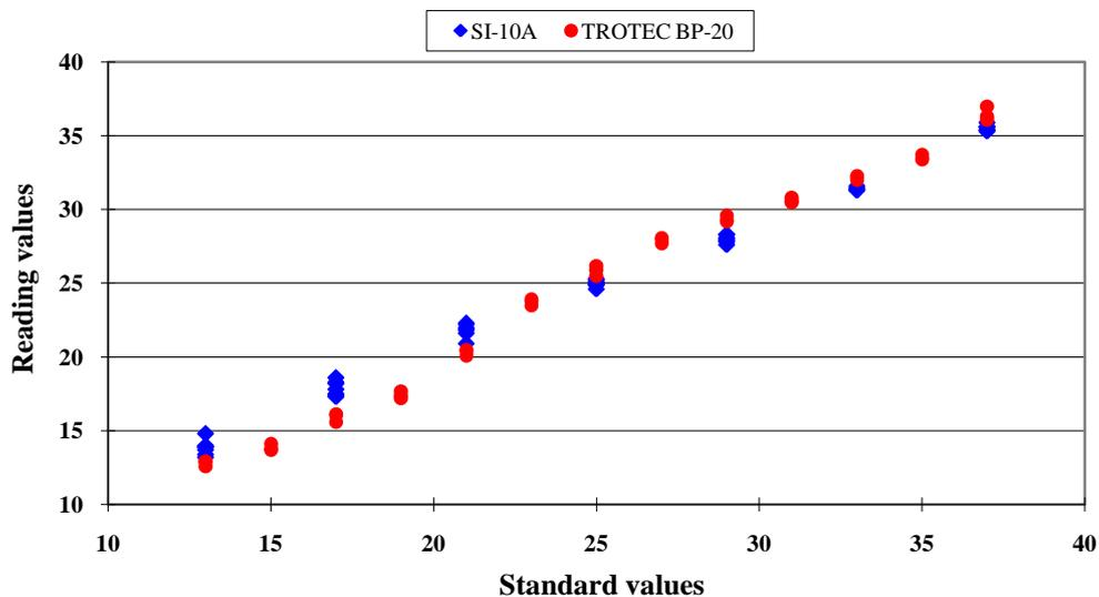
A nonlinear distribution of the data scattering was found. The error distribution of the Sentron SI-10A is shown in Figure 2.
