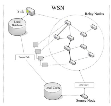
Figure 4. An illustration of the FSPC algorithm for secure data collection.
