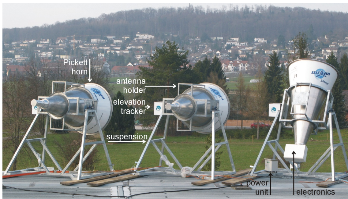
Figure 1. The ELBARA II systems mounted above the test site at the Swiss Federal Research Institute WSL, with the radiometer electronics and the power unit installed in the unit on the right.
