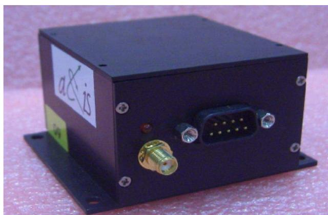
The output signals are addressed to a PC in the form of separate packets of data, so that the number and type of sensing channels can be set before the acquisition. Furthermore, the frequency at which data are transmitted from the IMU to the host can also be changed according to the specific
