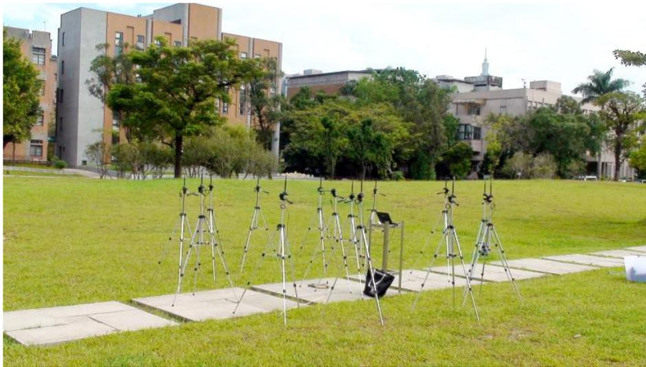
In real-world scenarios, it is impossible to construct a reference standard pattern for a reference node under all of the possible distances and orientations of the external antenna. We measured the values of RSSI when a sensor node is moved away from the reference node by five individual distances (1.8 m, 5 m, 10 m, 13 m, and 18 m).
