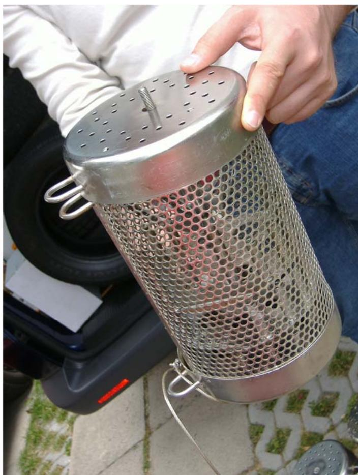
One passive sampler (Figure 4), a semi-permeable membrane device (SPMD), was placed at each site for one month in spring (May 7–June 4) and autumn (September 17–October 15). Semi-permeable membrane device sampler consists of a horizontal thin-walled tub from nonporous low density polyethylene, filled with synthetic lipid (triolein). The SPMD were commercially manufactured (Exposmeter AB, Sweden). After exposure the sampler membranes were rinsed briefly
