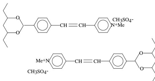
**Figure 1.** PVA-SbQ photocrosslinkable polymer.
