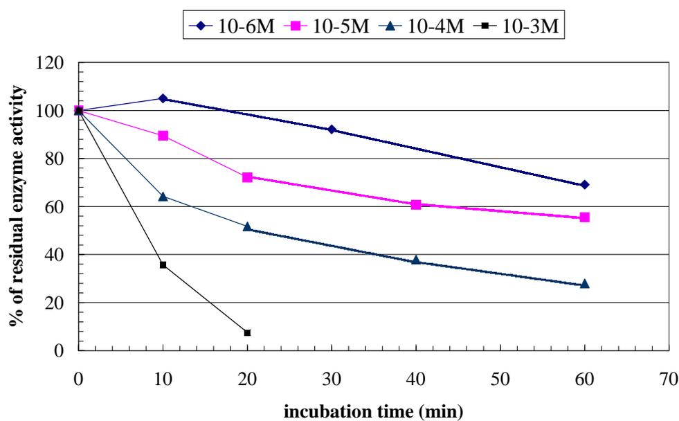
**Figure 2.** Inhibition effect on the BuChE-BSA FET sensor by trichlorfon. Percent of residual enzyme activity as a function of incubation time.
