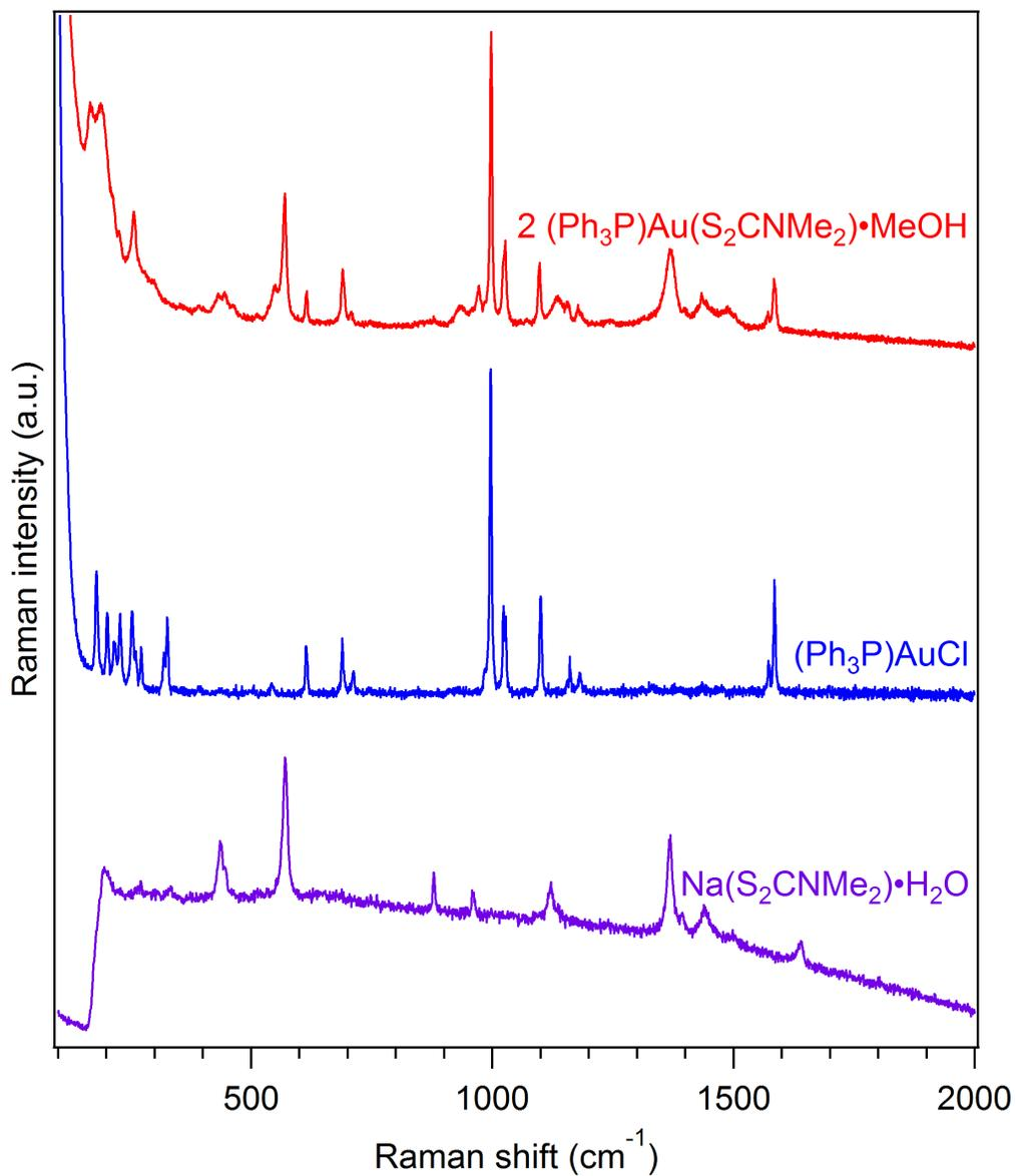
Figure S1. Raman spectra of the synthesized compound 2 (Ph<sub>3</sub>P)Au(S<sub>2</sub>CNMe<sub>2</sub>)•CH<sub>3</sub>OH and of its precursors. Raman spectra were measured at room temperature with an excitation wavelength of 785 nm are offset along the vertical axis for clarity.
