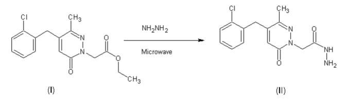
To (0.96 g, 3 mmol) of ethyl [4-(2-chlorobenzyl)-3-methyl-6-oxopyridazin-1(6H)-yl)] acetate (I), was added 10 ml of hydrazine hydrate. The mixture was placed in a pyrex tube which was then introduced into a Maxidigest MX 350 Prolabo microwave[4] monomode reactor and refluxed for 10 min on 60 w as irradiation power. After cooling, the product precipitates, and then is recristallised in absolute ethanol, yield : 80 % of (II) solid.
