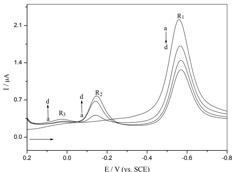
**Figure 6.** Differential pulse voltammograms using DNA-modified GCE in 0.10 M pH 4.5 acetate buffer containing  $1.0 \times 10^{-5}$  M *o*-nitrophenol before (a) and after reduction (b) by successive differential pulse voltammetry scans (10) from 0 to -0.8 V and (c) at constant potential  $E_d = -0.60$  V for  $t_d = 2$  minutes. (d) Differential pulse voltammogram obtained with the DNA-modified GCE in 0.10 M pH 4.5 acetate buffer.
