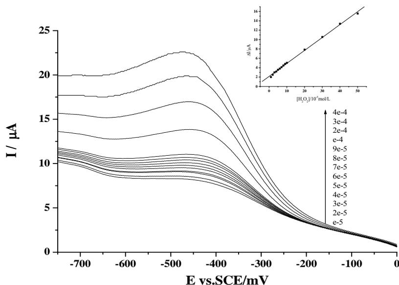
**Figure 2.** Voltammograms of the reduction peak obtained at a Hb-HY modified electrode for pH 7.0 Tris-HCl buffer with the additions of different concentrations of  $\text{H}_2\text{O}_2$ . Inset is plots of the reduction peak current against  $\text{H}_2\text{O}_2$  concentration. Scan rate:  $200 \text{ mV s}^{-1}$ . For the Hb-HY modified electrode preparation, the HY and Hb concentrations are separately  $1 \times 10^{-2} \text{ mol/L}$  and  $6.20 \times 10^{-5} \text{ mol/L}$ .
