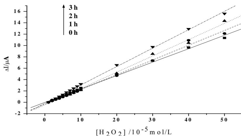
**Figure 3.** Linear relationship between the increase of the reduction peak current and  $\text{H}_2\text{O}_2$  concentration after visible light irradiation of 0h, 1h, 2h, 3h, respectively (The value of the reduction peak with  $10^{-5} \text{ mol/L}$   $\text{H}_2\text{O}_2$  is set as 0). Others same as in Figure 2.
