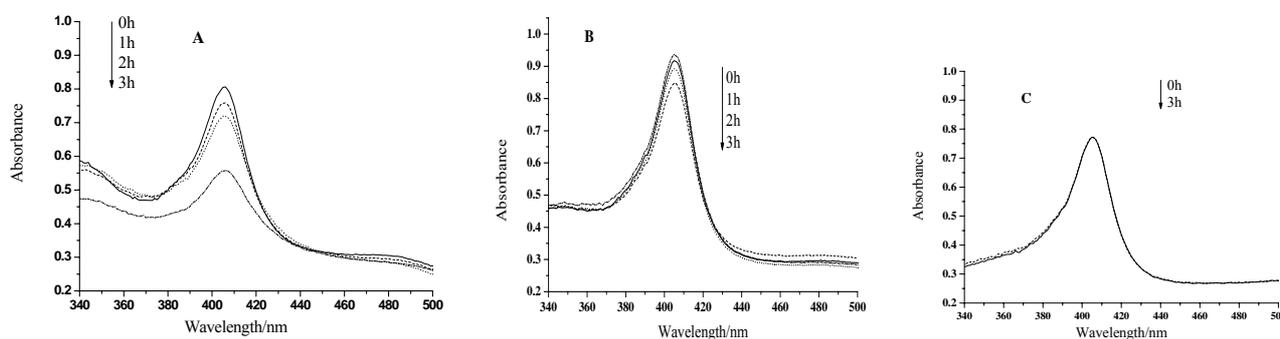
**Figure 1.** (A) UV-vis spectra of hemoglobin mixed with HY after visible light irradiation for 0h, 1h, 2h, 3h, respectively. HY concentration:  $5 \times 10^{-4}$  mol/L. Hb concentration:  $3.10 \times 10^{-6}$  mol/L. (B) is the case for HY concentration of  $2.5 \times 10^{-4}$  mol/L. (C) is the case for the absence of HY.
