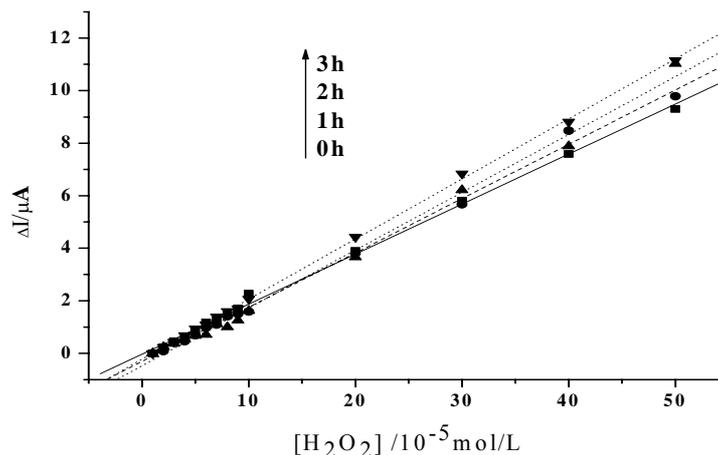
**Figure 4.** Linear relationship between the increase of the reduction peak current and  $\text{H}_2\text{O}_2$  concentration after visible light irradiation of 0h, 1h, 2h, 3h, respectively. HY concentration:  $5 \times 10^{-3}$  mol/L. Others same as in Figure 3.
