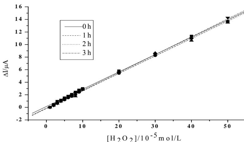
**Figure 5.** Linear relationship between the increase of the reduction peak current and  $\text{H}_2\text{O}_2$  concentration after visible light irradiation of 0h, 1h, 2h, 3h, respectively in an anaerobic condition. Others same as in Figure 3.
