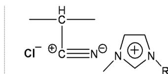
**Figure 8.** The interaction between PAN and [BMIM]Cl.
