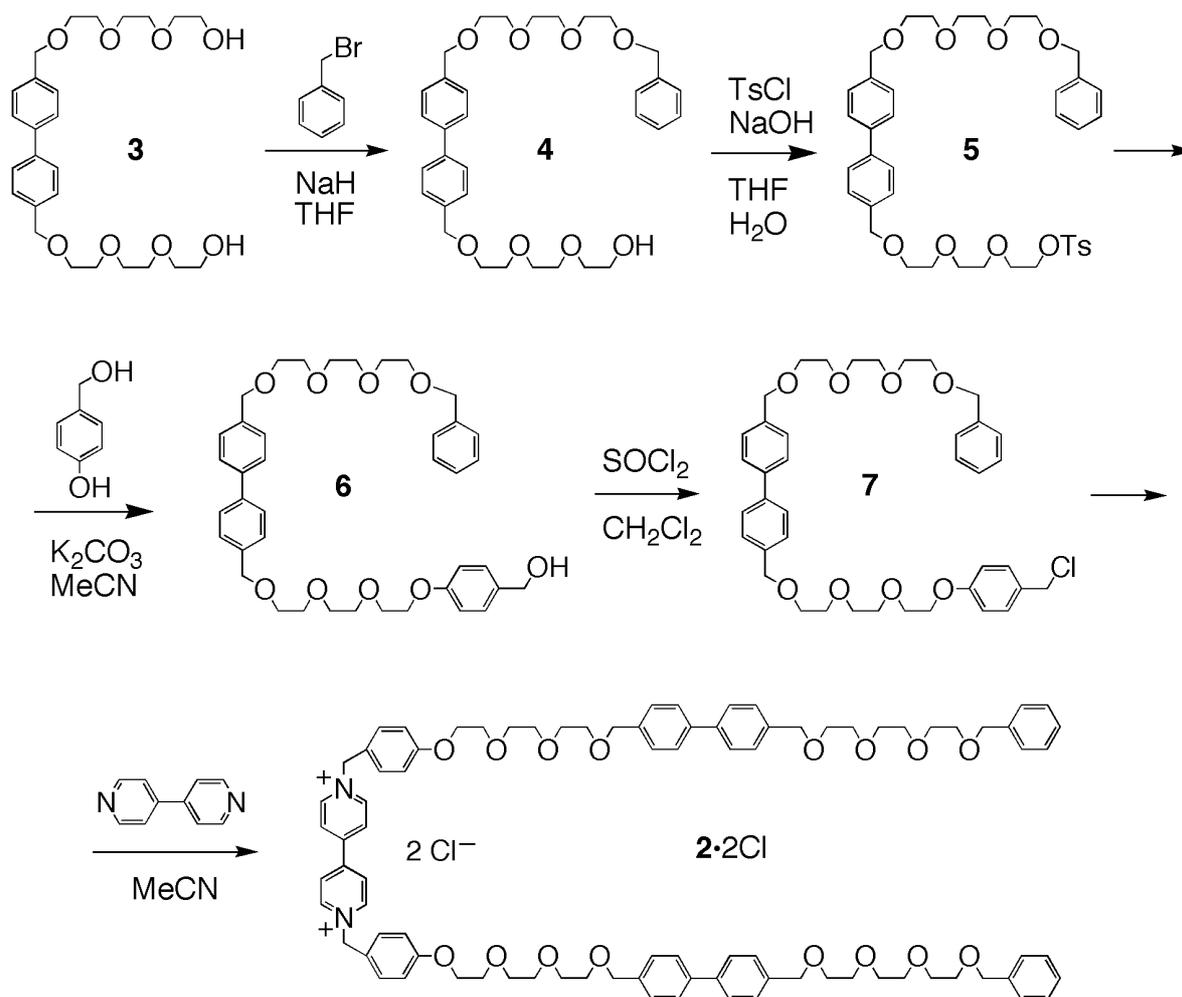
**Scheme 1.** Synthesis of the linear component **2·2Cl**.
