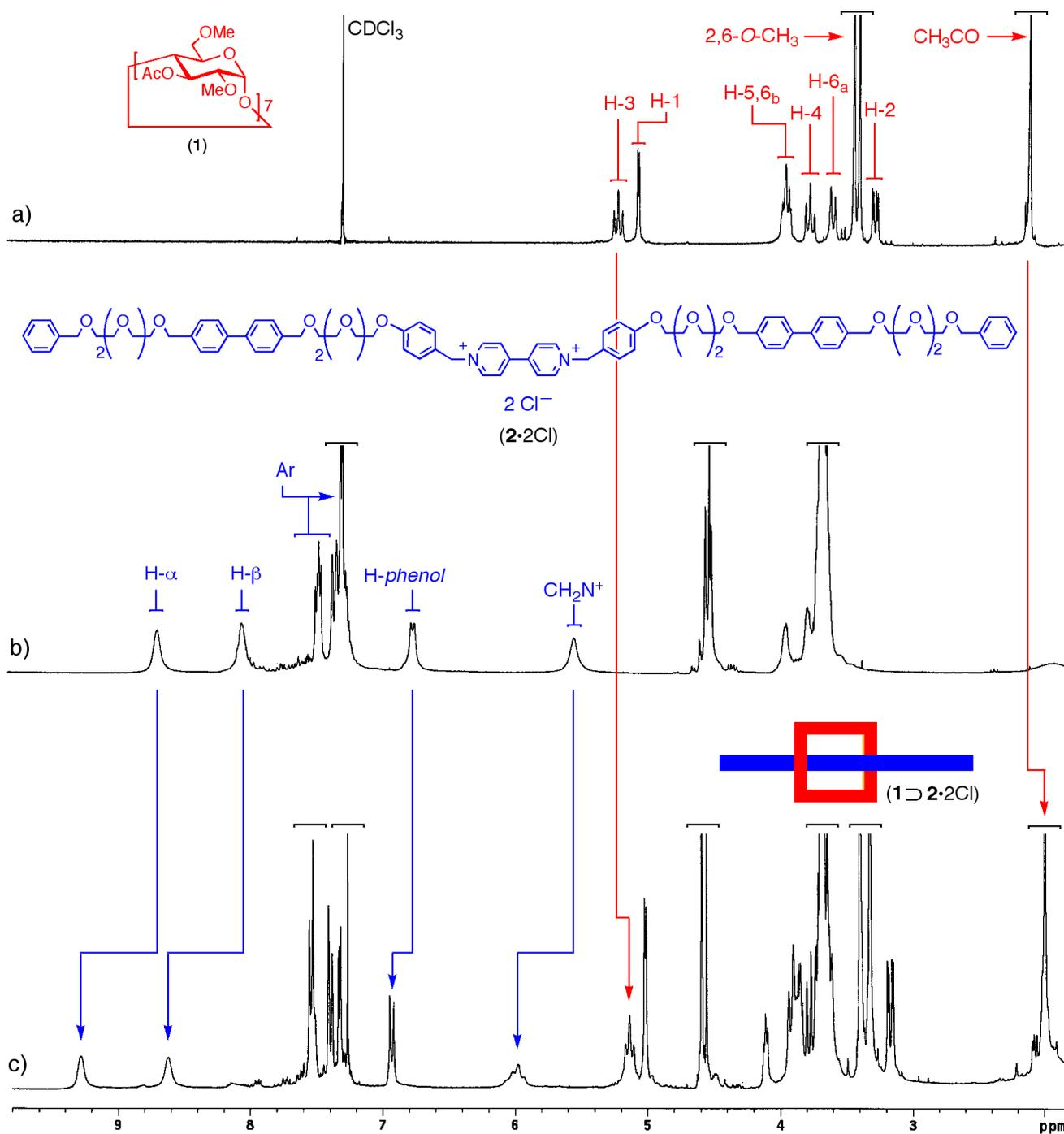
**Figure 2.**  $^1\text{H}$  NMR spectra (300 MHz,  $\text{CDCl}_3$ , 22 °C) of 5 mM samples of: a) cyclodextrin **1**; b) linear component **2·2Cl**; c) [2]pseudorotaxane **1⊃2·2Cl**.
