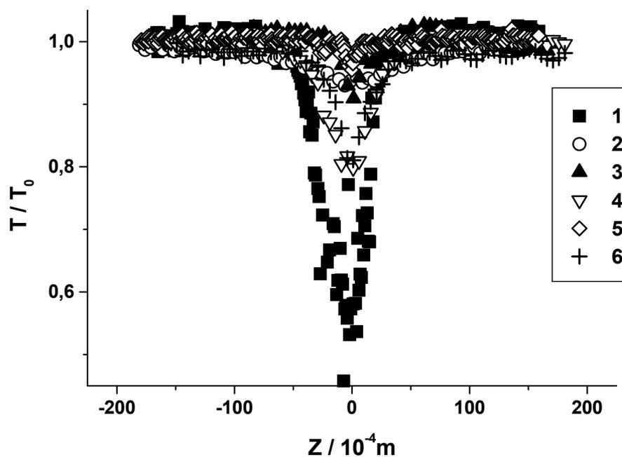
**Figure 1.** Z-scan profiles for the species (1)-(6). The species were irradiated at the same level. The linear transmittance  $T_0$  of the examined solutions was 0.9. The concentrations were in the range  $4\text{-}5 \cdot 10^{-5}$  M. The 1-chloronaphthalene solvent didn't show any NLO behavior at the used level of irradiation.
