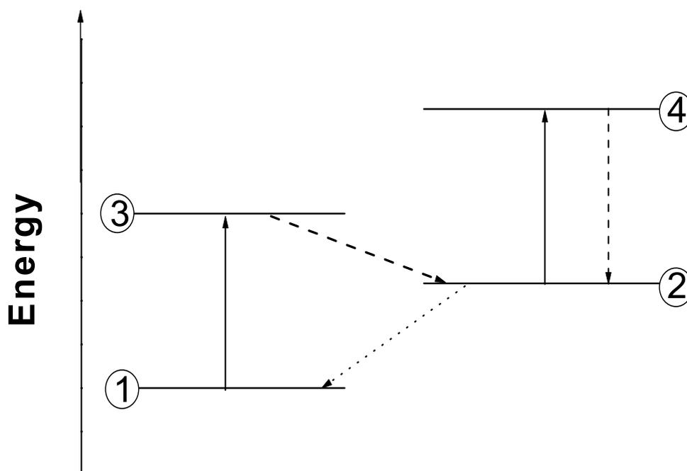
**Figure 2.** Energy diagram of a four-level system. Full lines indicate absorption from singlet ground [1→3] and triplet excited states [2→4]; dashed lines represent intersystem crossing [3→2] and excited state fluorescence [4→2]; dotted line indicates phosphorescence [2→1].
