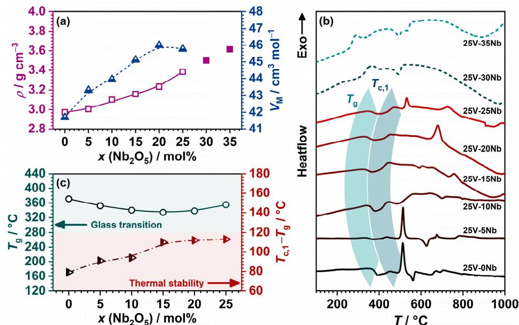
**Figure 1.** (a) Dependence of density,  $\rho$ , and molar volume,  $V_M$ , on Nb<sub>2</sub>O<sub>5</sub> content; (b) DTA curves; and (c) dependence of glass transition temperature,  $T_g$ , and the parameter ( $T_c - T_g$ ) on Nb<sub>2</sub>O<sub>5</sub> content. The lines connecting data points in (a,c) are a guide for the eye.
