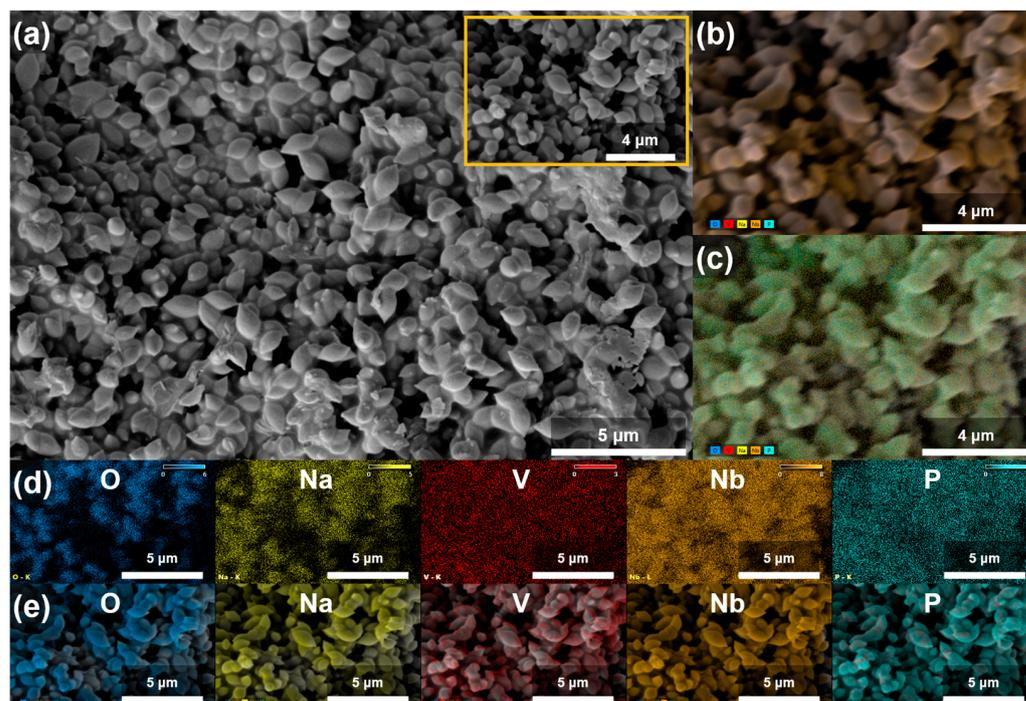
**Figure 3.** (a) SEM micrographs of 25V-30Nb glass–ceramic; (b) count X-ray mapping; (c) quantitative X-ray mapping; (d) count and (e) quantitative elemental mapping of O, Na, V, Nb, and P from a selected area of the given glass–ceramic.
