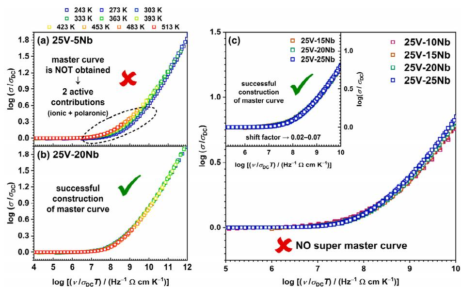
**Figure 7.** Summerfield scaling of conductivity spectra of (a) 25V-5Nb glass and (b) 25V-20Nb glass. (c) Construction of super master curve of the conductivity isotherms obtained by applying the Summerfield scaling procedure to all the investigated glasses; inset: individual master curves of glasses with  $10 \leq x \leq 25$  shifted along the x-axis to overlap with the reference master curve of 25V-10Nb glass.
