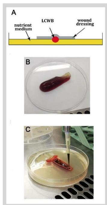
**Figure 2.** Lubbock chronic wound biofilm model: (A) schematic representation of the treatment of LCWB transferred to artificial wound bed, adapted from Kucera et al. [60]; (B) mature LCWB of *S. aureus* and *P. aeruginosa* grown together; (C) antimicrobial application in a LCWB model located in an artificial wound bed.
