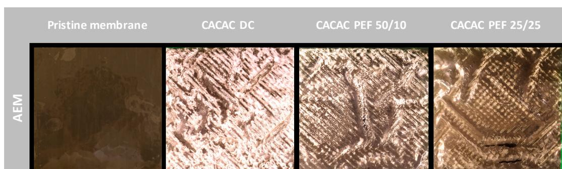
**Figure 5.** Entire anion-exchange membranes' (AEMs') anode sides (10 cm<sup>2</sup>) photographs before and after ED for all three current conditions. AEM comprised of A1 and A2 with no visible differences.
