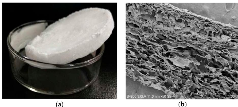
**Figure 2.** Sponge appearance (digital camera) (a) and internal structure (scanning electron microscope) (b).
