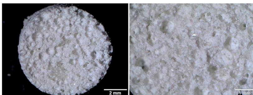
**Figure 3.** Microstructure of the chitosan-agarose-HA (chit/aga/HA) scaffold visualized by a stereoscopic microscope.
