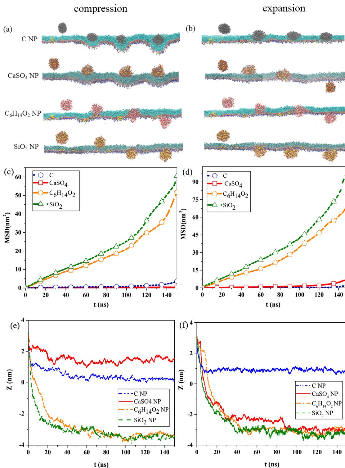
**Figure 1.** Interaction between nanoparticles (NPs) and the pulmonary surfactant monolayer. Snapshots of the interaction in the (a) exhalation and (b) inhalation breathing states; mean-square displacements (MSDs) of the NPs in (c) exhalation and (d) inhalation breathing states; centroid-to-centroid distance between the NPs and monolayer in (e) exhalation and (f) inhalation breathing states.
