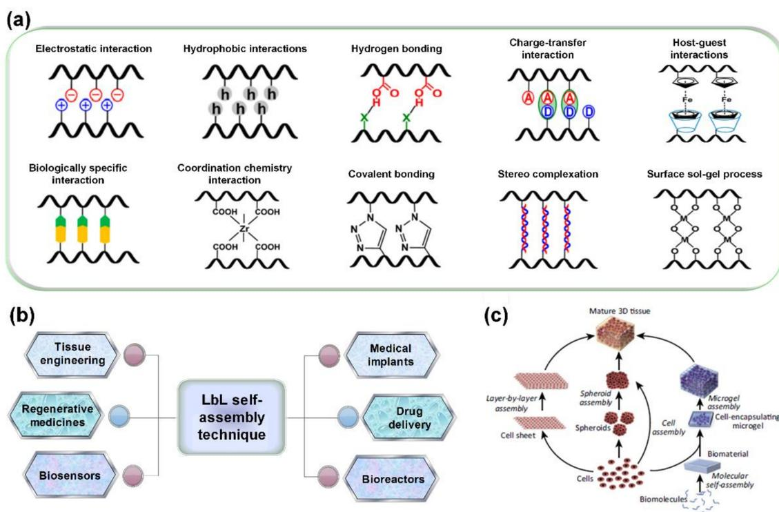
**Figure 2.** (a) Molecular interactions driving the LbL self-assembly of materials; (b) schematic showing the main biomedical application fields for LbL self-assembly technique; (c) schematic of multiscale assembly strategies for engineering tissue constructs. Reprinted from [18,56] with permissions from American Chemical Society and Elsevier.
