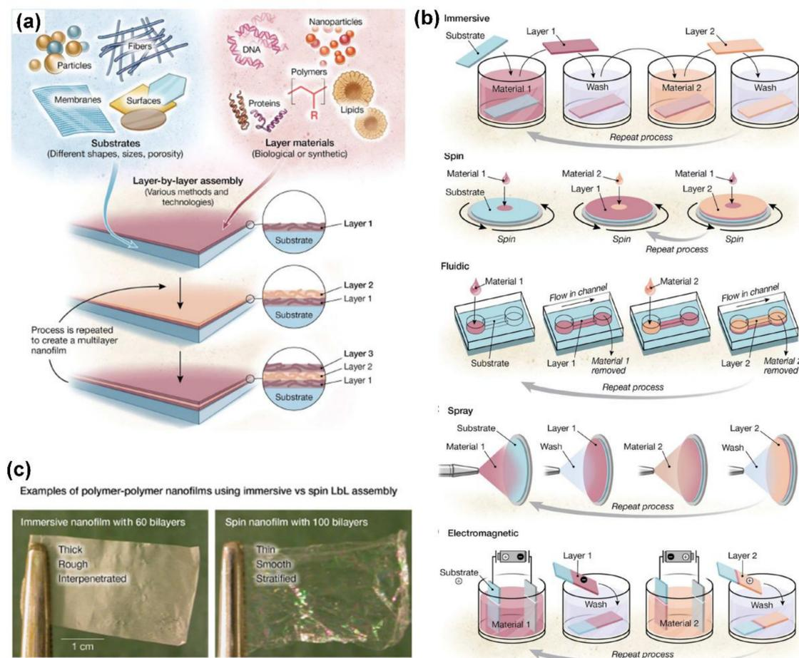
**Figure 1.** (a) Schematic overview of LbL assembly technique with fabrication capacity on any type of substrates and from an extensive choice of materials; (b) schematics showing the five main technology categories for LbL assembly; (c) a typical comparison of different films using immersive and spin assembly. Reprinted from [17] with permission from American Association for the Advancement of Science.
