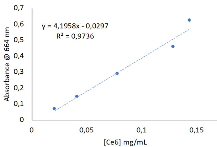
**Figure S2.** Chlorin-e6 calibration curve.
