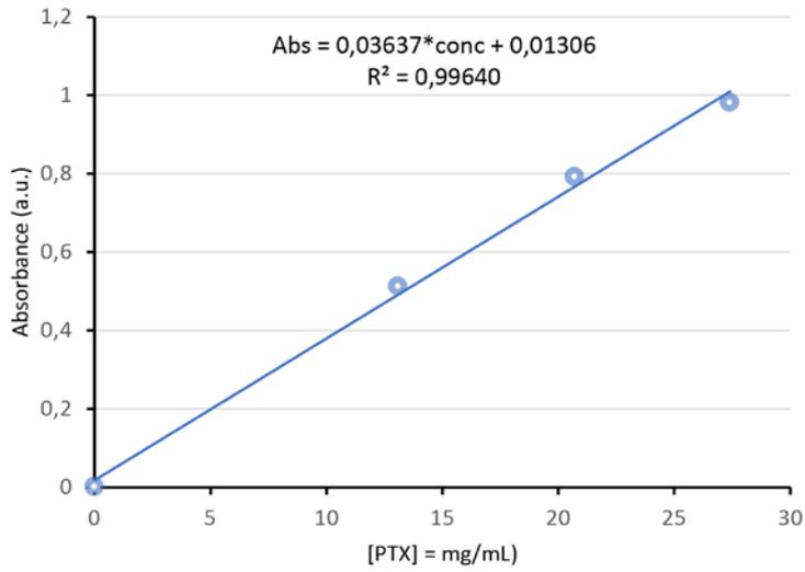
**Figure S3.** PTX calibration curve.
