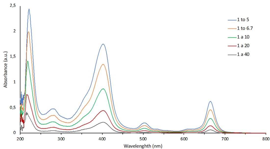
**Figure S1.** Absorbance spectra of chlorin-e6 solution at different Ce6 concentrations.
