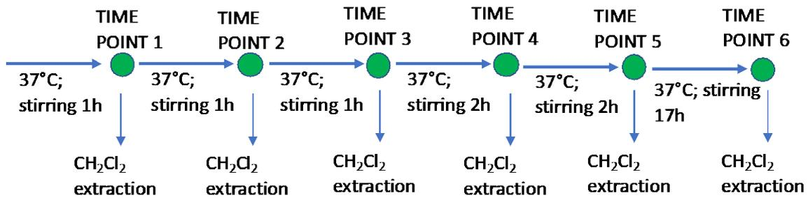
**Figure S4.** Graphical flow chart of the protocol used to evaluate PTX release over time.
